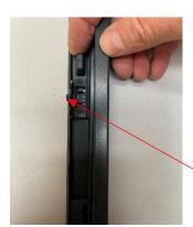
On the left and right uprights on the frame, you will find 4 sliding bracket carriers (2 on each side) these are movable so the brackets can be lined up with the bracket slots on the corresponding Perfect Fit blind when assembled.
