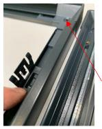
This picture shows the Universal frame lying next to the assembled Perfect Fit blind, and the bracket is being slid in line with the slot in the Perfect Fit frame. When all 4 brackets are lined up the Universal frame is ready to be screwed to the cabin side around the window opening
