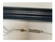
At the bottom of the frame, connect the hook to the spring, this will put the required tension into the blind.
